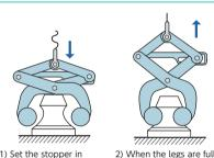
1) Set the stopper in release position, lower the clamp so that the legs of the tongs properly fit into the bank block neck.
