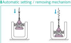
2) Hoist down until the wire rope is completely loosened.
