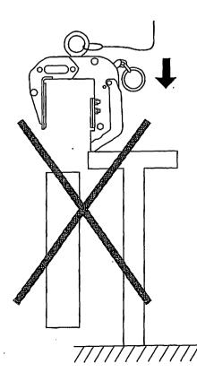
8. Be careful not to catch the remote control ropes on obstacles such as scaffoldings during lifting and hanging. (The lock lever will be opened and the clamp may come off, leading to falling accidents.)
