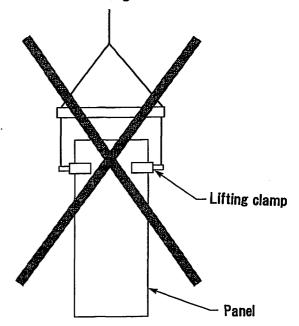
7. Do not hit lifting clamp or lifting load to other objects during lifting.(Be careful especially during hanging.)Impact or loose rope may cause falling accidents.
