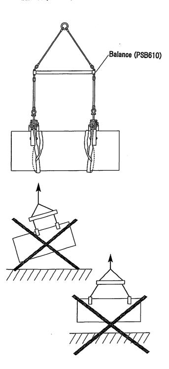
Do not lift more than two plates simultaneously.
