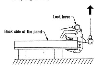
14. When lifting the molded plate in the upright direction, make sure that the frame column is on the surface of the clamp pad. Clamping the part where there's no frame column may cause damage or falling of the panel.
