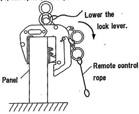
Check the clamping range before proceeding to the next operation. Repeat from the procedure No. 3.
