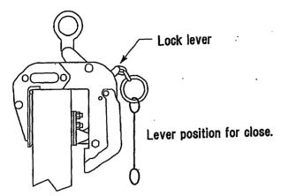
6. The clamp main body has a hook for mounting the sling belt for double safety. Use it for safer operation. This is a subsidiary hook part for safety. Do not use it by itself.
