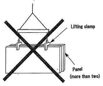
Do not lift the panel with side gripping.
