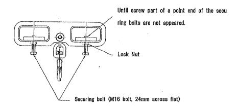
(2) Place the lifting clamp on the roper rest (sleeper etc.)
