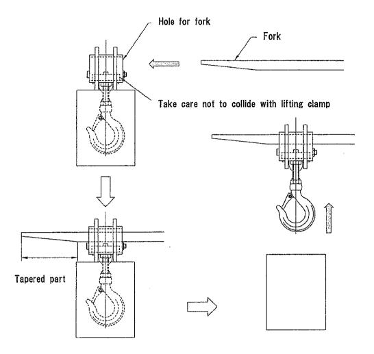
(5) Tighten the lifting clamp and forks of the fork lift by securing bolts (The angle of the forks of the fork lift must be horizontal at this time) Never use when the fork of the fork lift is not horizontal.
