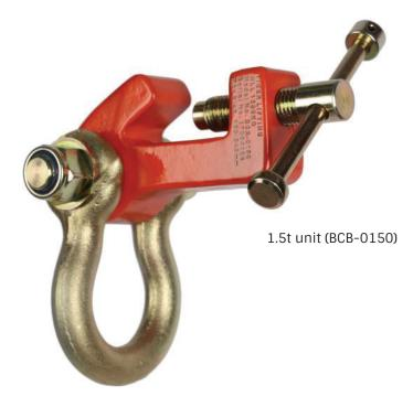
Our BCB bulb flat bar anchor can be side loaded up to 45° and cross loaded up to 15° without derating the unit, while still maintaining a 4:1 factor of safety.
